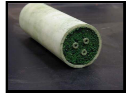
Thermocouple protection system for gasifier application [2].
